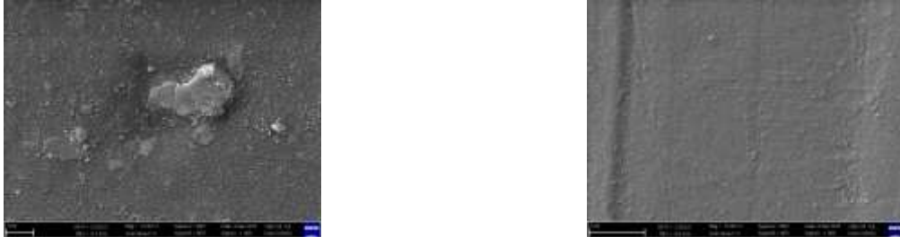
Fig. 3 The difference in the structure of the surface left) before and right) after applying the impregnation (magnification 10 000x)
