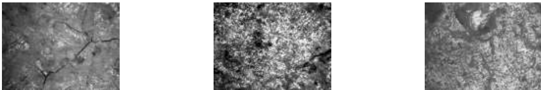
Fig. 7 200°C left) untreated sample, middle) pure emulsion, right) emulsion with nanoparticles
