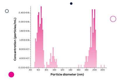
The above graph shows a single sample comprising three distinct subpopulations of particles, with known mean diameters of 61 nm, 95 nm and 195 nm. These particles were isolated using a qEVoriginal 20 nm column and subsequently analysed using an NP100 on the Exoid.
