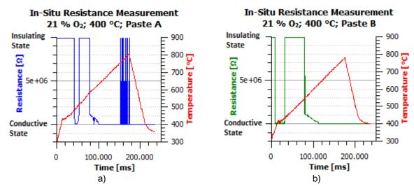
**Fig. 5** The dependence of resistance on the temperature using Profile 400.
