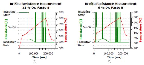
Fig. 4 The dependence of resistance on the temperature and the content of O2 for the paste B.
