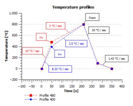
Fig. 2 Used temperature profiles.
