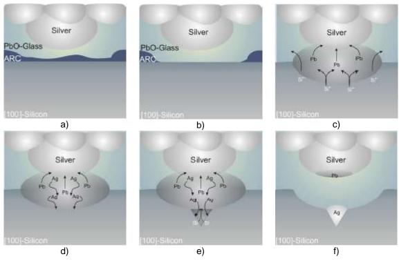
**Fig. 1** Simplified model of contact formation: a) schematic cross section of Ag thick film paste on [100] Si after combustion of organics; b) glass etches through SiN<sub>x</sub> layer; c) redox reaction between Si and glass, lead (Pb) is formed; d) liquid Pb starts to melt Ag; e) Ag - Pb melt reacts with Si, inverted pyramids are formed; f) on cooling down Ag recrystallises on (111)-Si planes [5].
