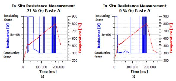
Fig. 3 The dependence of resistance on the temperature and the content of O₂ for the paste A.
