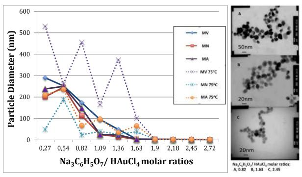
**Fig. 2** Average particle diameter changes and different morphologies for gold nanoparticles with different Na<sub>3</sub>C<sub>6</sub>H<sub>5</sub>O<sub>7</sub>/Au molar ratios via citrate reduction method (**right:** particles mean diameters evaluated by Nanotrac wave analyser, **left:** TEM images of the synthesized gold nanoparticles)
