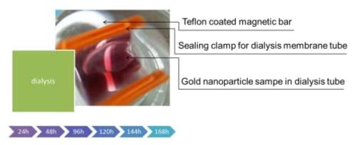
Fig. 1 Scheme purification processes for gold nanoparticles in this study
