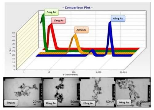
Fig. 3 Particle size distribution and different morphologies for gold nanoparticles via citrate reduction method with different Au concentrations (from 5mg to 40mg Au/100ml) (right: particles size distribution evaluated by Nanotrac wave analyser, left: TEM images of the synthesized gold nanoparticles)
