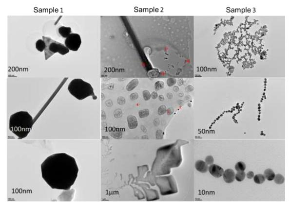
Fig. 4 Different morphologies of gold nanoparticles via NaBH<sub>4</sub> reduction method with different reaction parameters (TEM analysis) **Sample 1:** with high reaction rate, **Sample 2:** with modified reaction rate, **Sample 3:** with controlled low reaction rate.
