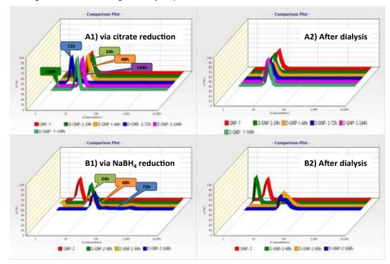
Fig. 5 Gold nanoparticle changes after dialysis experiment through time evaluated by Nanotrac wave analyzer (A: gold nanoparticle synthesized via citrate reduction method, B: gold nanoparticles synthesized via NaBH<sub>4</sub> reduction method)
